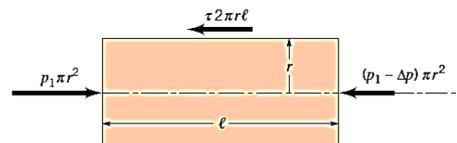
**Gambar 2.2. Diagram Benda Bebas Elemen Fluida**
